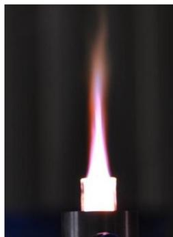
Figure 2. An actual image of the atmospheric microwave plasma jet at an argon gas flow rate of 6 lpm and microwave forward power of 2000 W. The plasma flame is contained in a quartz
