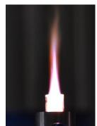
Figure 2. An actual image of the atmospheric microwave plasma jet at an argon gas flow rate of 6 lpm and microwave forward power of 2000 W. The plasma flame is contained in a quartz
