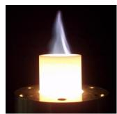
Figure 1. An actual image of the atmospheric microwave plasma jet at an argon gas flow rate of 6 lpm and microwave forward power of 600 W. The plasma filaments are contained in an alumina tube.
